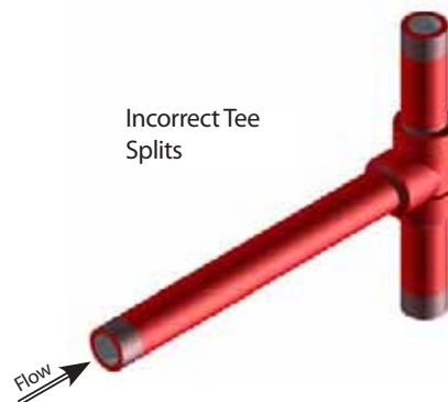
Figure 44 - Bull tee orientation "incorrect"
