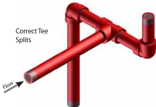
Figure 43 - Bull tee orientation "correct"
