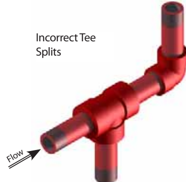
Figure 44 - Bull tee orientation "incorrect"
